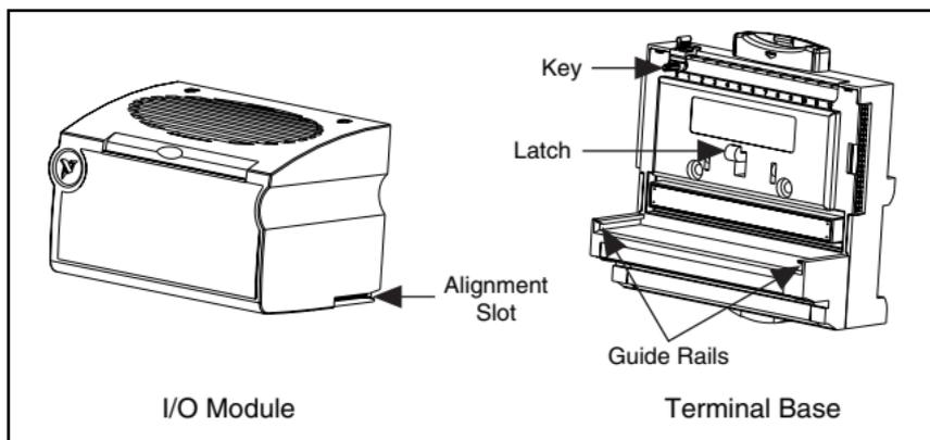
**Figure 1.** Installing the FP-AO-210
