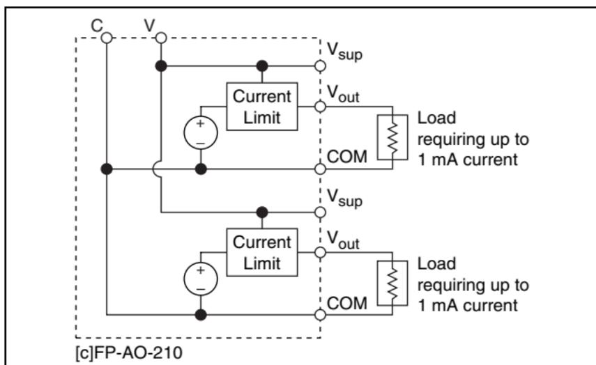
**Figure 3.** Two Loads without External Supply
