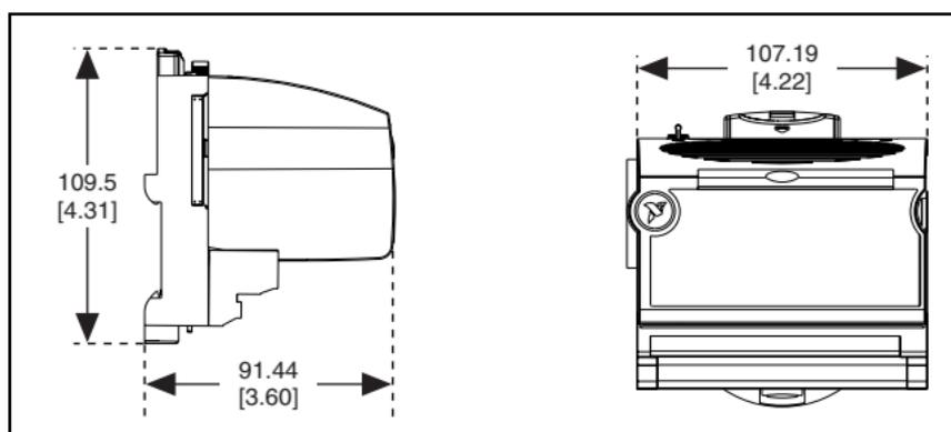
**Figure 6.** FP-AO-210 Mechanical Dimensions
