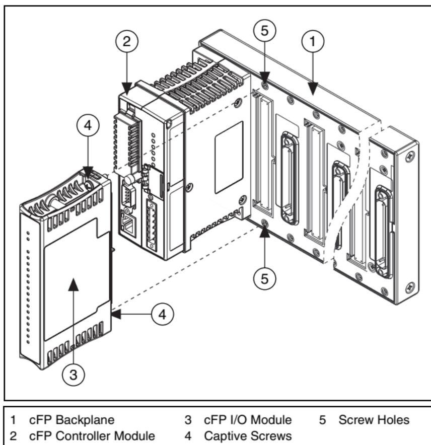
**Figure 2.** Installing the cFP-AO-210
