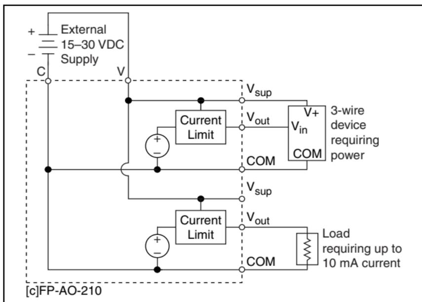
**Figure 4.** Two Loads with External Supply
