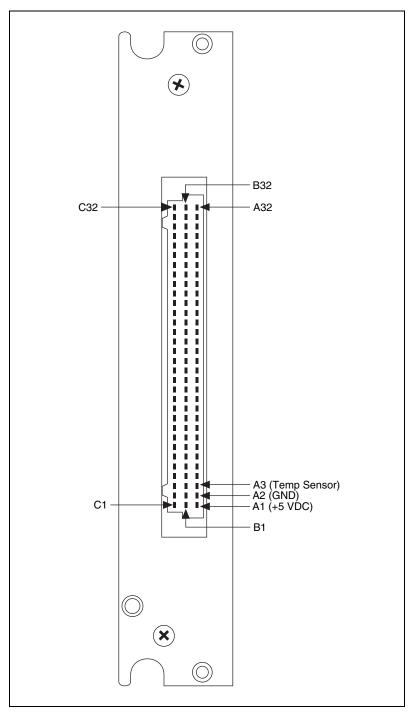
Figure 1. SCXI-1303 Front Connector Pin Assignments
