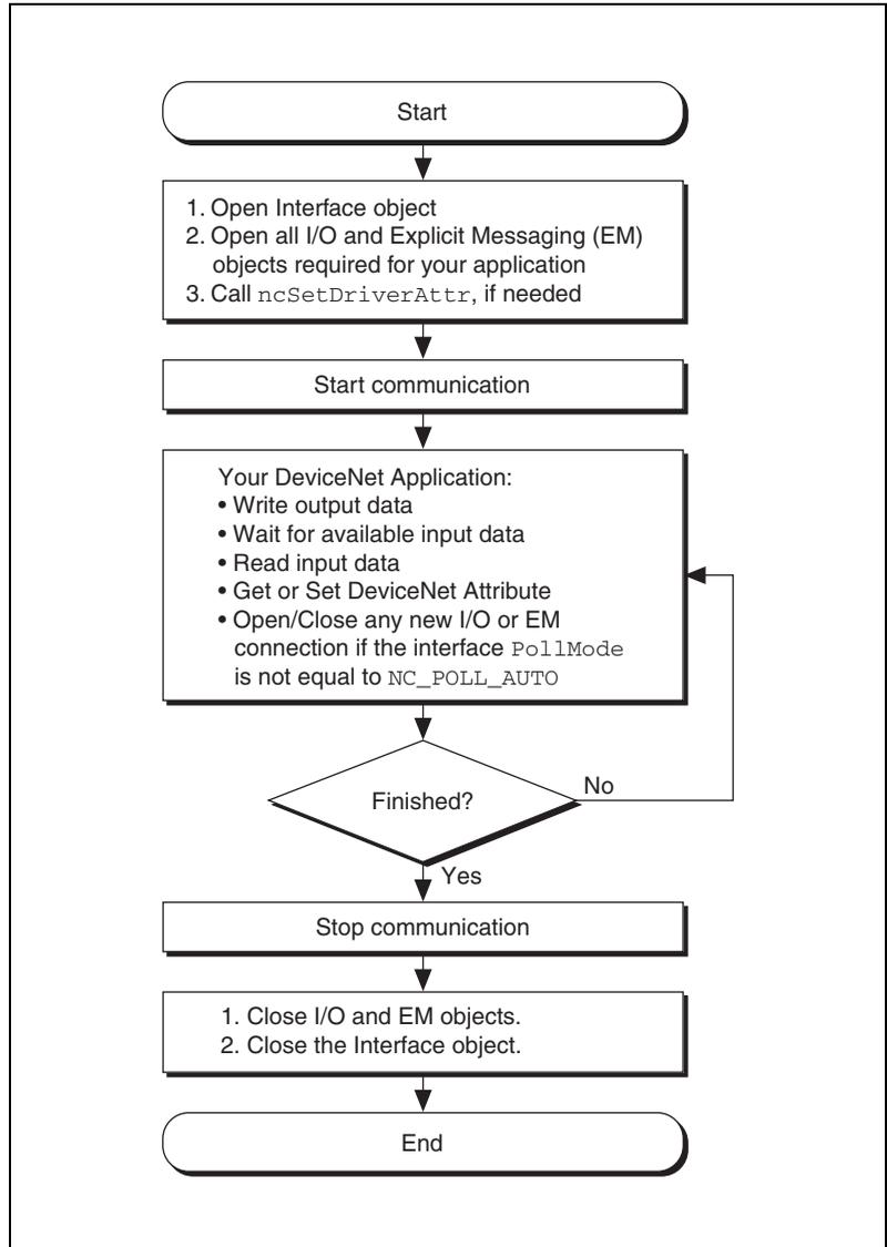
**Figure 3-1.** General Programming Steps for an NI-DNET Application
