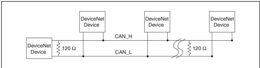
**Figure B-7.** Termination Resistor Placement
