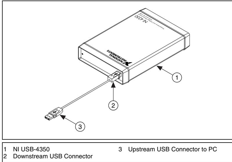
**Figure 2.** NI USB-4350 with USB Cable
