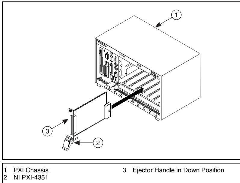
**Figure 3.** NI PXI-4351 with PXI Chassis
