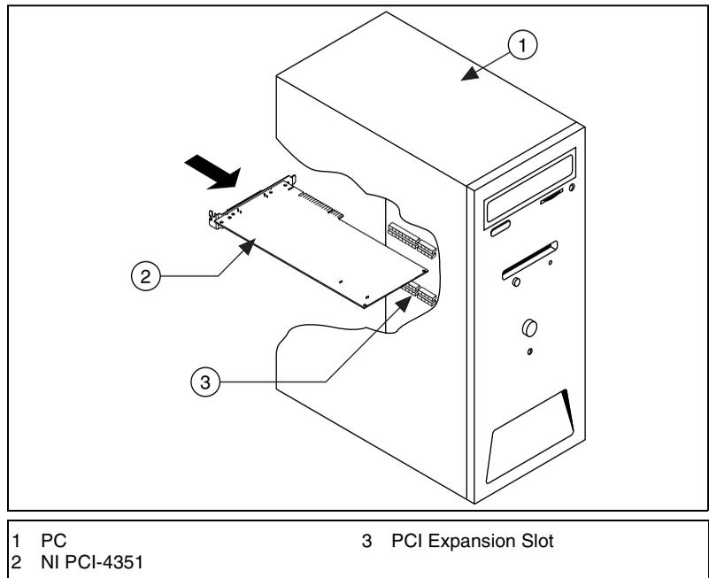
**Figure 4.** NI PCI-4351 with PC
