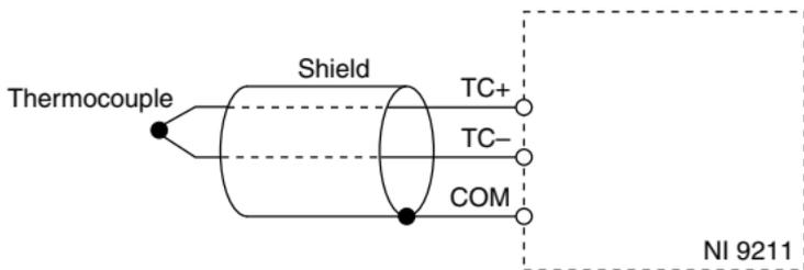
Connect the COM terminal to a common-mode voltage reference on the thermocouple. A valid common-mode voltage reference is a voltage that is within  $\pm 1.5$  V of the common-mode voltage of the thermocouple
