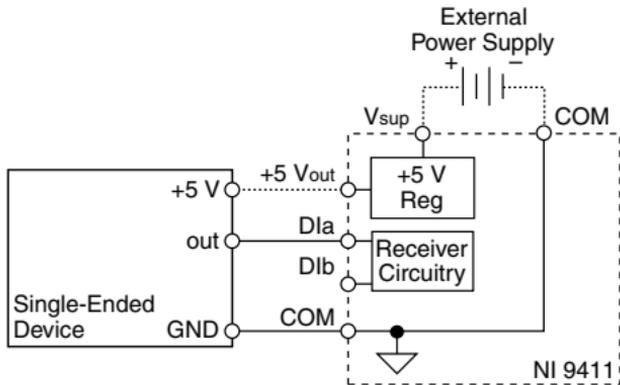
The NI 9411 compares the difference between DIa and COM to the digital logic levels to determine if the signal is in the high range or low range.
