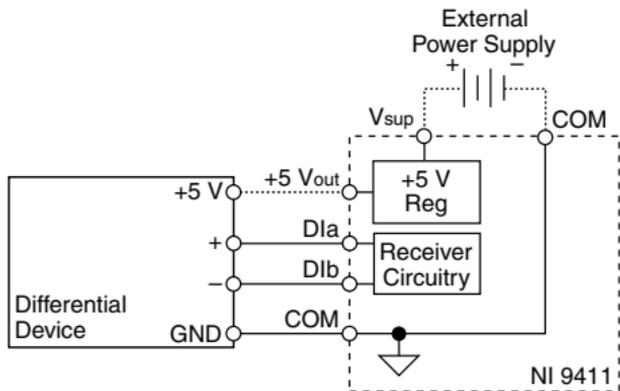
The NI 9411 compares the difference between DIa and DIb to the digital logic levels to determine if the signal is in the high range or low range.
