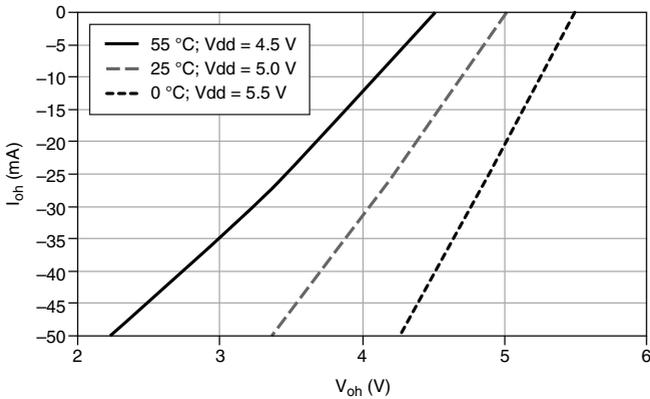
**Figure 5.** PFI <0..15>/P1/P2: I<sub>oh</sub> versus V<sub>oh</sub>
