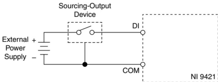
The NI 9421 channel registers as ON when the sourcing-output device applies a voltage or drives a current that is in the input ON range to DI. The channel registers as OFF when the device applies a voltage or drives a current that is in the input OFF range to DI. If no device is connected to DI, the channel registers as OFF.
