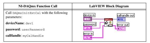
You use the object myCalHandle in all subsequent NI-DAQmx calibration function calls.
