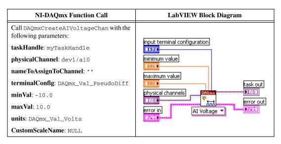
5. Modify the AI voltage channel property using the following functions.
