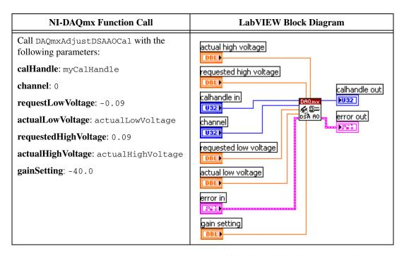
17. Repeat steps 4 through 16 for all remaining gain values used in steps 4 and 16. Also modify the device requested high and low voltages used in steps 4 and 16. You can find the values in Table 7.
