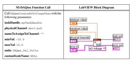
5. Modify the AO voltage channel property using the following functions.
