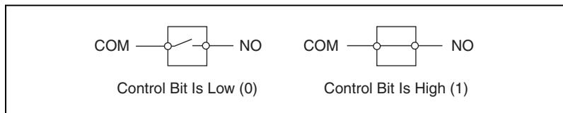
**Figure 4.** Programmable Power-Up States for Form A Relays
