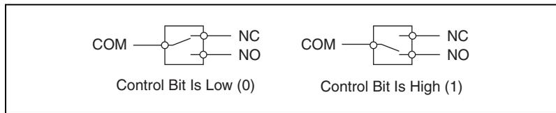
**Figure 3.** Programmable Power-Up States for Form C Relays
