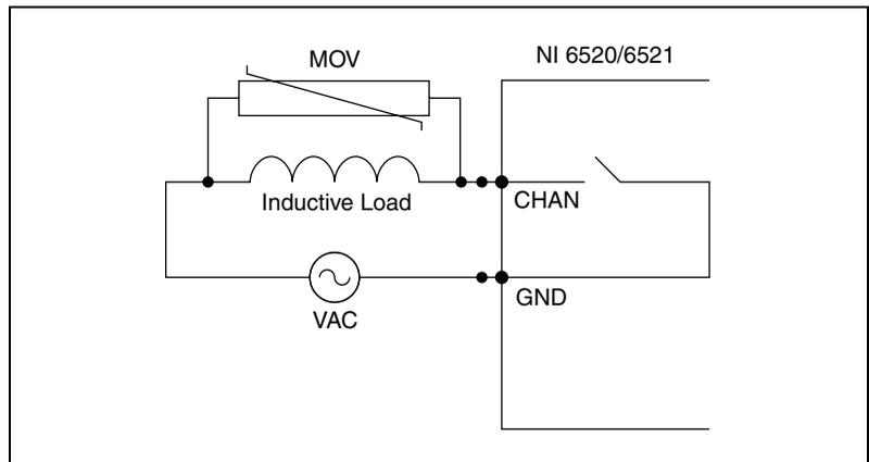
**Figure 13.** Contact Protection for AC Inductive Loads
