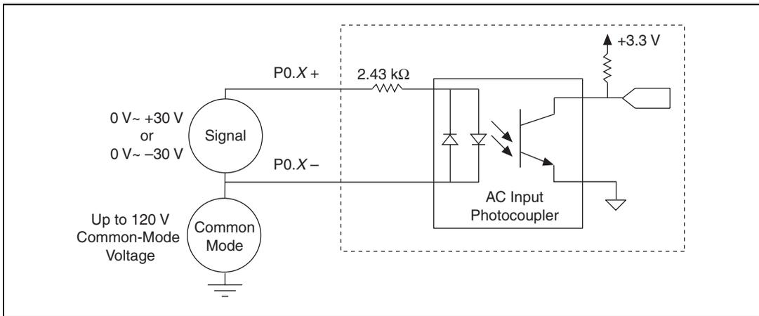
**Figure 7.** NI 6521 Input Signal Connection Example
