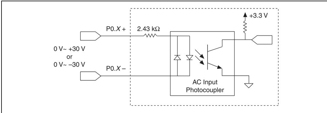
**Figure 6.** NI 6520 Input Signal Connection Example
