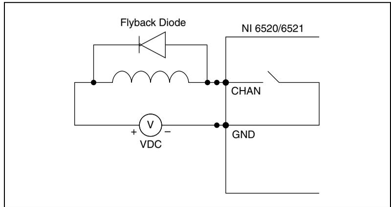
**Figure 12.** Contact Protection for DC Inductive Loads
