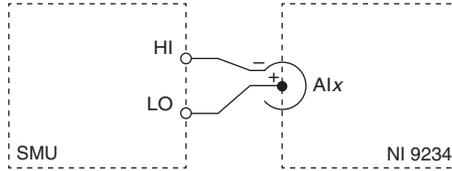
6. Configure the SMU as a current source and set the voltage limit to the lowest appropriate range to measure 24 V.
