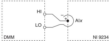
2. Configure the DMM for a DC current measurement in the lowest appropriate range to measure 2 mA.
