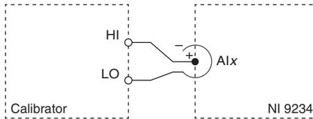
3. Verify that the calibrator output is not grounded (floating).
