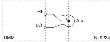
2. Configure the DMM for a DC current measurement in the lowest appropriate range to measure 2 mA.
