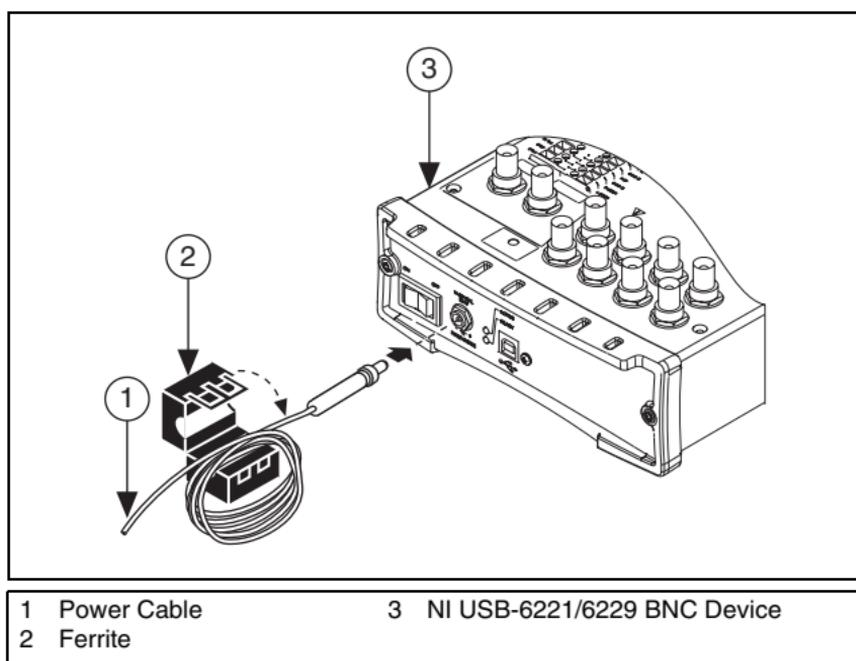
**Figure 1.** Installing the Ferrite on the Power Cable
