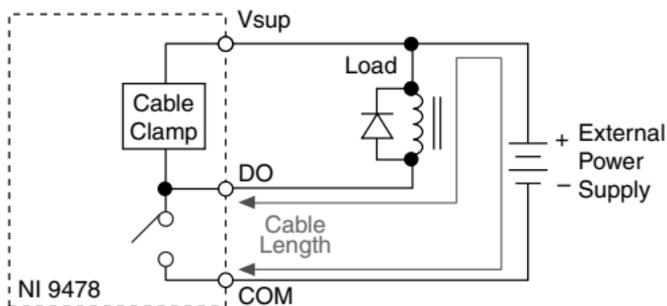
NI recommends adding a capacitor across the power supply leads and a diode from the DO lead to the Vsup lead. Connecting a capacitor and a diode reduces the effective cable length and dissipated heat.
