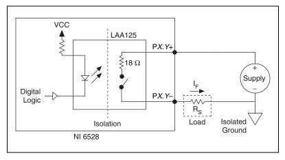
Figure 7. Sourcing Current Connection Example
