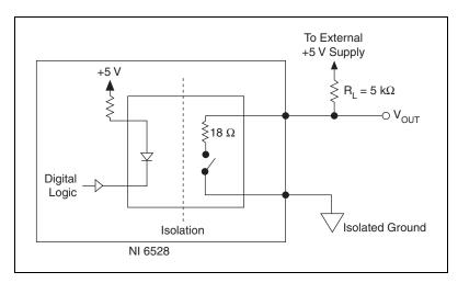
Figure 8. TTL-Level Device Connection Example
