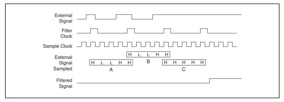
Figure 3. Digital Filtering Example
