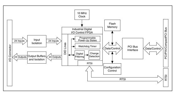
Figure 1. NI 6528 Block Diagram
