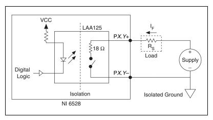
Figure 6. Sinking Current Connection Example
