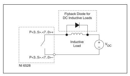
Figure 9. Limiting Flyback Voltages at the Inductive Load
