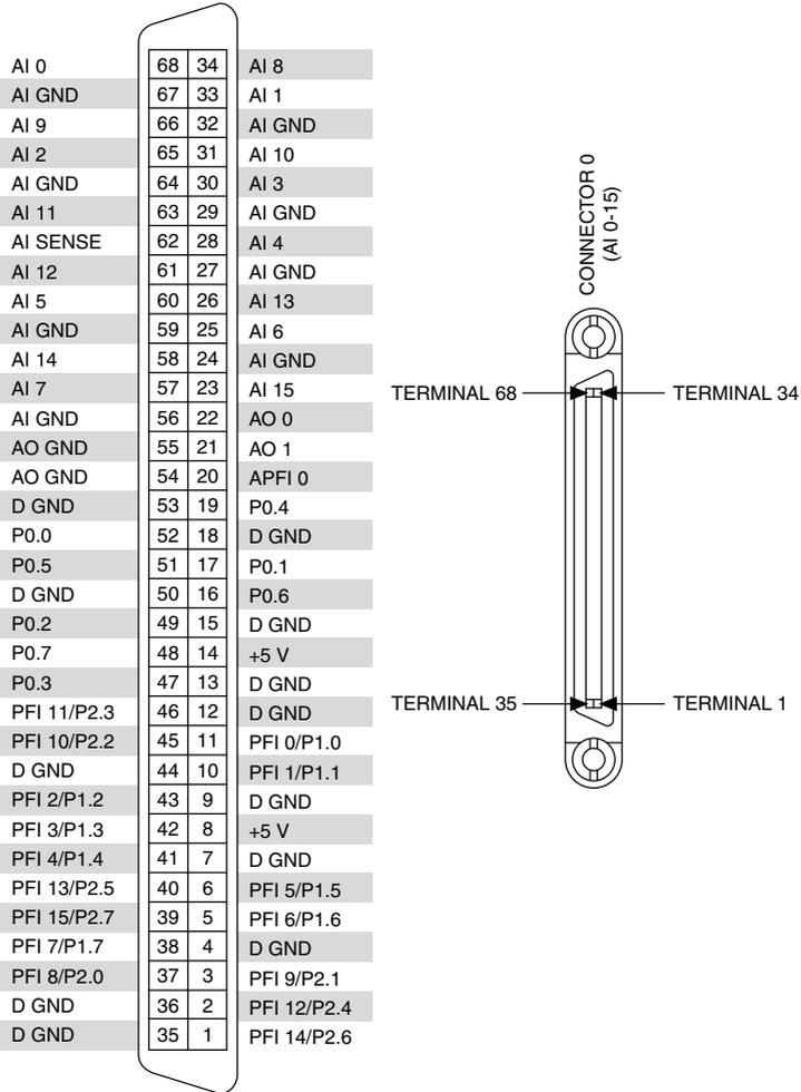
**Figure 10. NI USB-6251 Screw Terminal Pinout**
