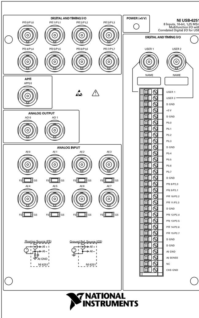
**Figure 12. NI USB-6251 Mass Termination Pinout**
