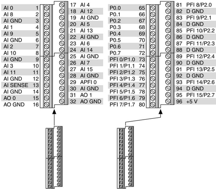
**Figure 11. NI USB-6251 BNC Front Panel and Pinout**
