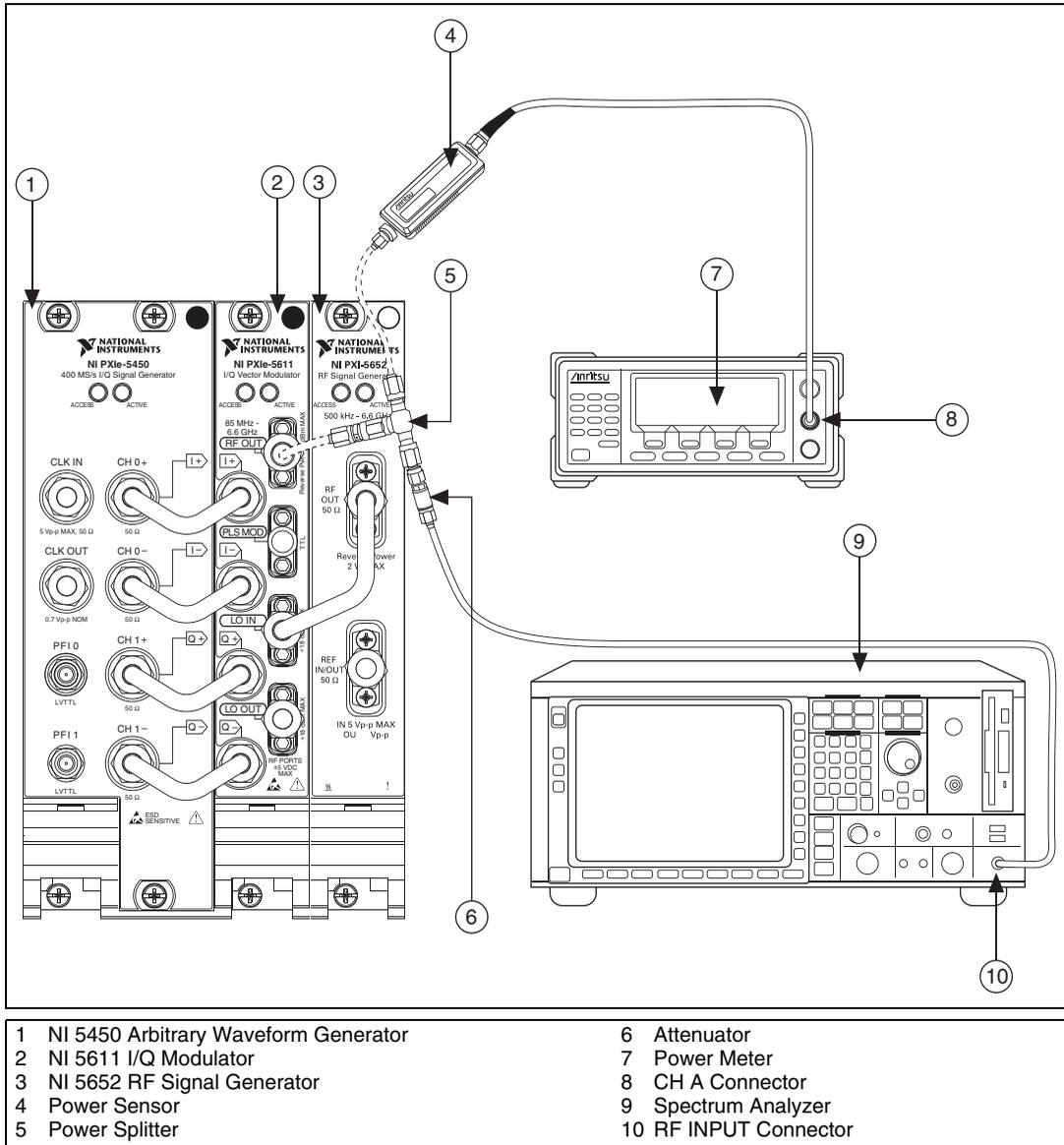
**Figure 4.** Connecting Hardware to Adjust RF Path Gain
