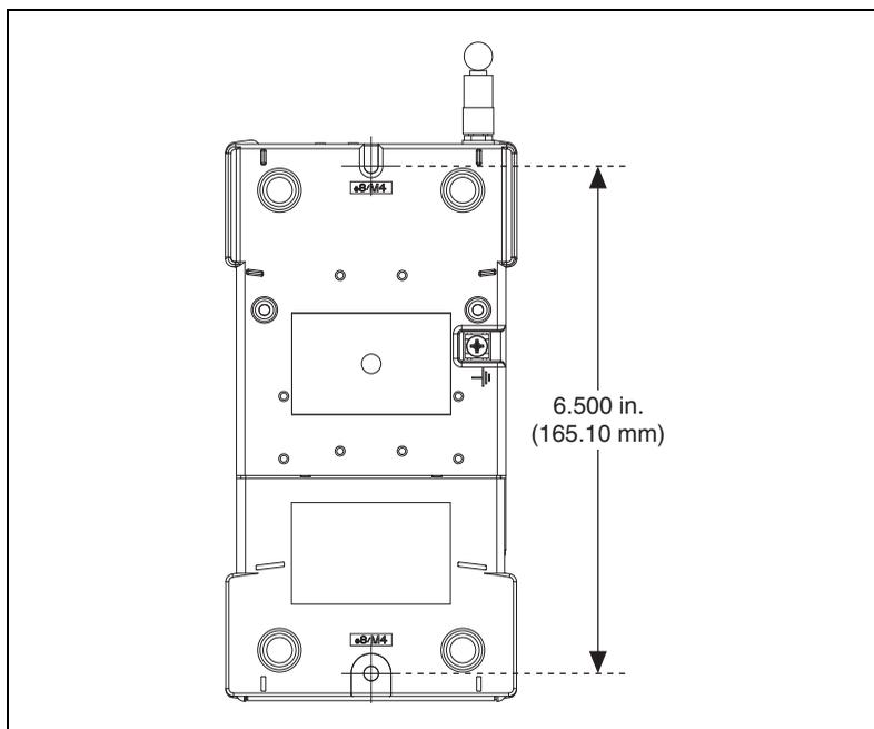
**Figure 5.** Device Panel Mounting Dimensions
