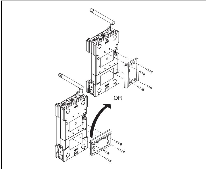
**Figure 4.** NI WLS/ENET-9000 Series Device DIN-Rail Installation
