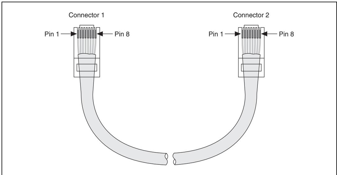
Figure 9. Ethernet Connector Pinout
