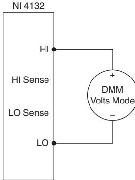
Table 2 lists the voltage set points that you must request and measure for each range to complete verification. For example, the 10 V range requires verification at 10 V, 0 V, and -10 V outputs from the NI 4132, taking measurements using the external DMM at each.
