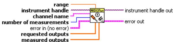
**Table 10.** NI-DCPower Cal Adjust Voltage Level VI/Function Parameter Descriptions
