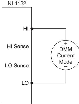
Table 3 lists the current set points that you must request and measure for each range to complete verification. For example, the 10  $\mu\text{A}$  range requires verification at 10  $\mu\text{A}$ , 0.2  $\mu\text{A}$ , -0.2  $\mu\text{A}$ , and -10  $\mu\text{A}$  outputs from the NI 4132, taking measurements using the external DMM at each point.
