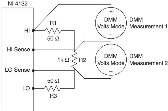
2. Connect the resistors to the HI and LO terminals on the NI 4132 as shown in Figure 5. Connect the remote sense leads directly across the 1 kΩ resistor (R<sub>2</sub>).
