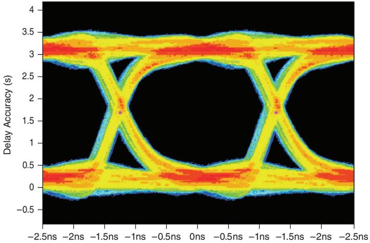
Figure 3 shows an eye diagram of a 400 Mbps PRBS waveform in DDR mode at 3.3 V. This waveform was captured on DIO 0 at room temperature into 50  $\Omega$  termination.
