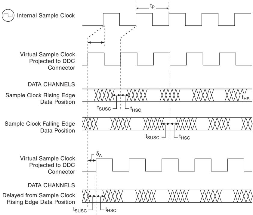
$t_{DDCSC}$  : Time Delay from DDC Connector to Internal Sample Clock
