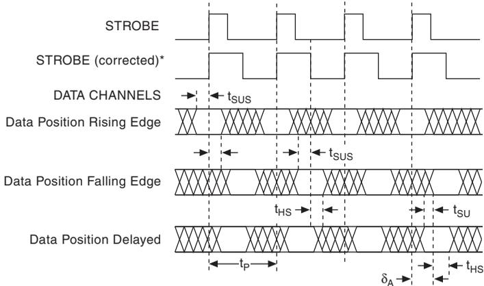
$t_{SUS}$  = Set-Up Time to STROBE
