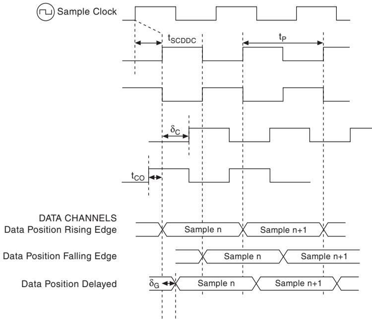
$t_{SCDDC}$  : Time Delay from Sample Clock (Internal) to DDC Connector
