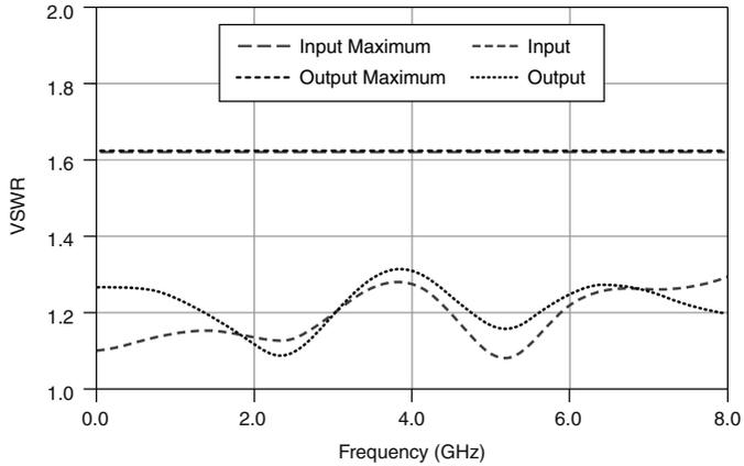
**Figure 8.** Measured Input and Output VSWR at 31.5 dB Attenuation Setting
