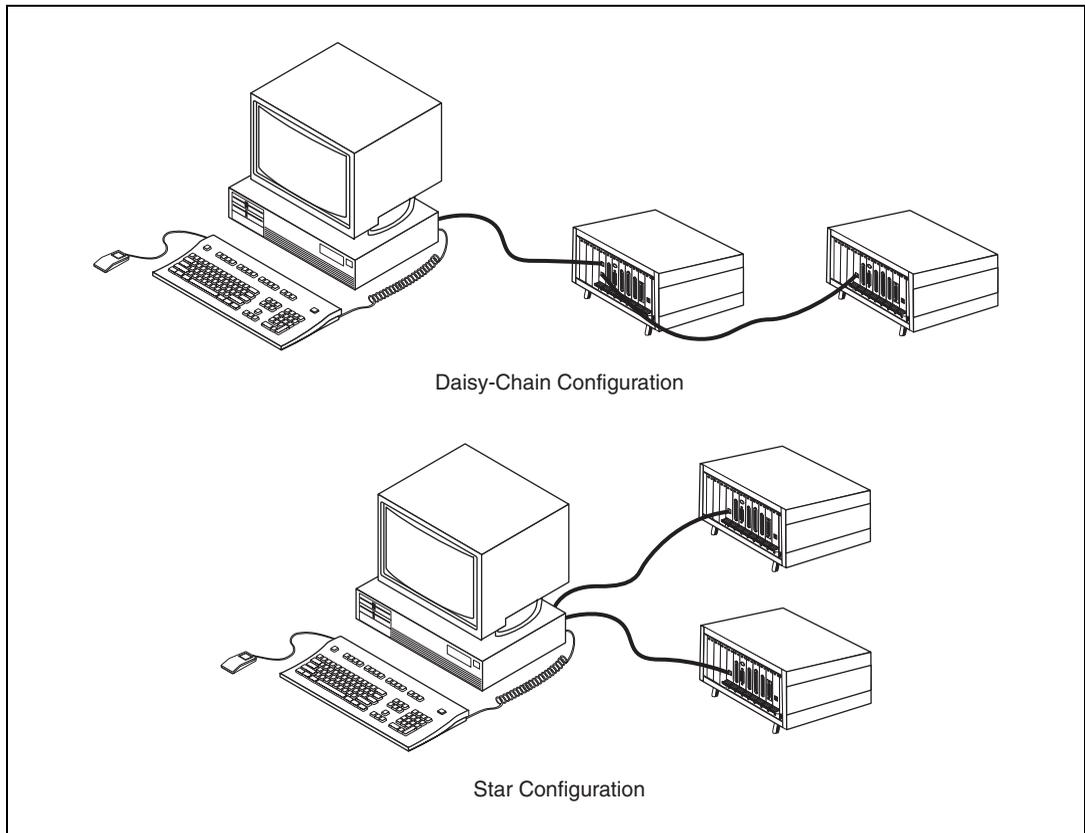
**Figure 1-2.** Topologies for Fiber-Optic MXI-Express x4 Configuration
