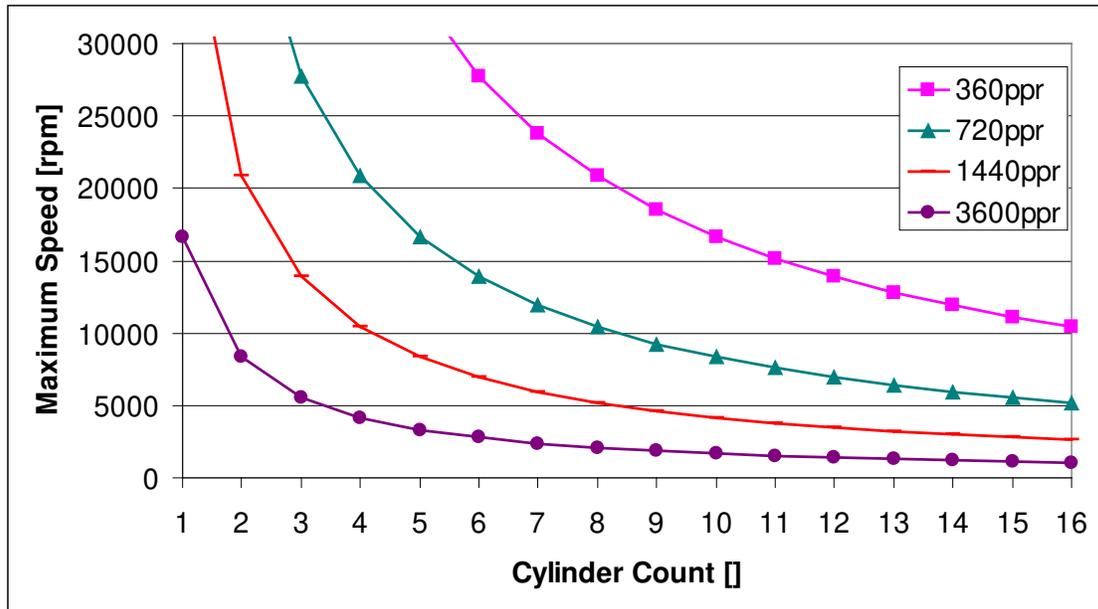
Figure 33: Maximum Engine Speed (USB-6251 & USB-6259)
