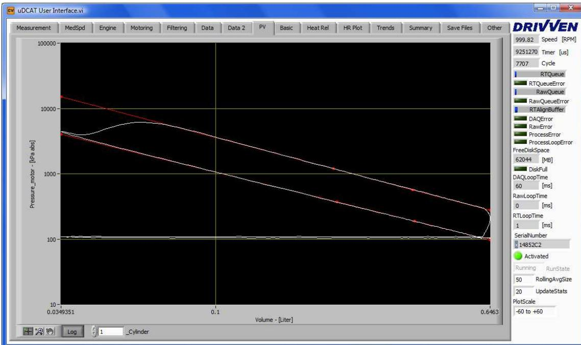
Figure 14: PV Diagram
