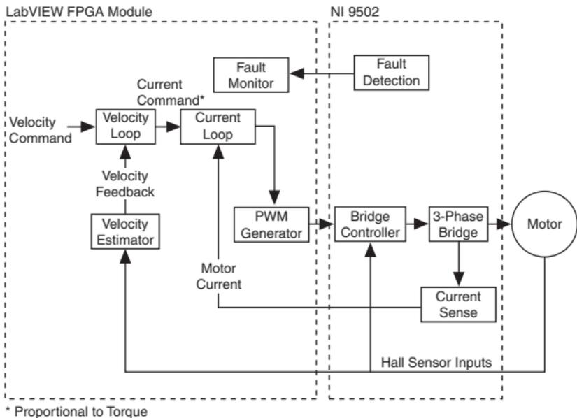
Figure 2 shows the NI 9502 working with the LabVIEW FPGA module in FOC commutation mode.
