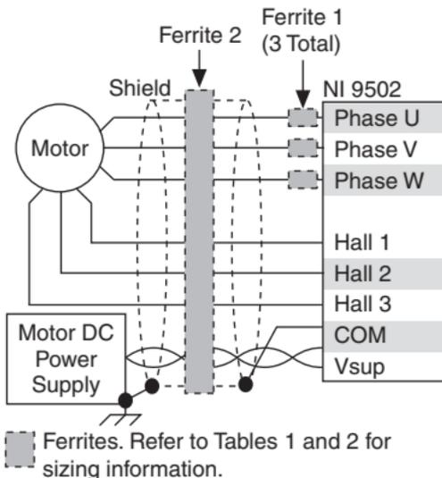
**Figure 6.** NI 9502 Cable Connection (Two Cable Option)
