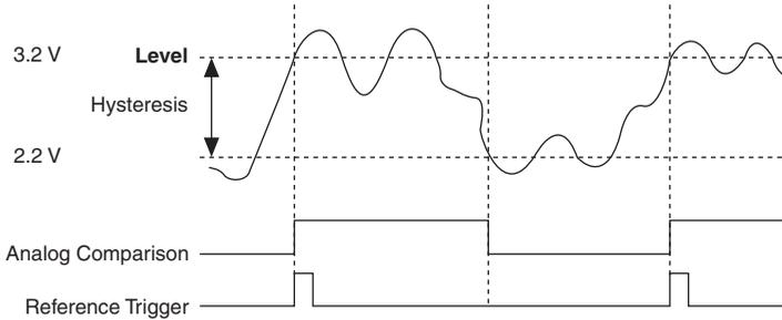
When using hysteresis with a falling slope, the trigger is armed when the signal starts above Level, plus the hysteresis value, and asserts when the signal crosses below Level. For example, if you add a hysteresis of 1 V to a level of 3.2 V, the signal must start at or rise above 4.2 V to arm the trigger. The trigger asserts as the signal falls below 3.2 V and deasserts when it rises above 4.2 V, as shown in Figure 2-14.
