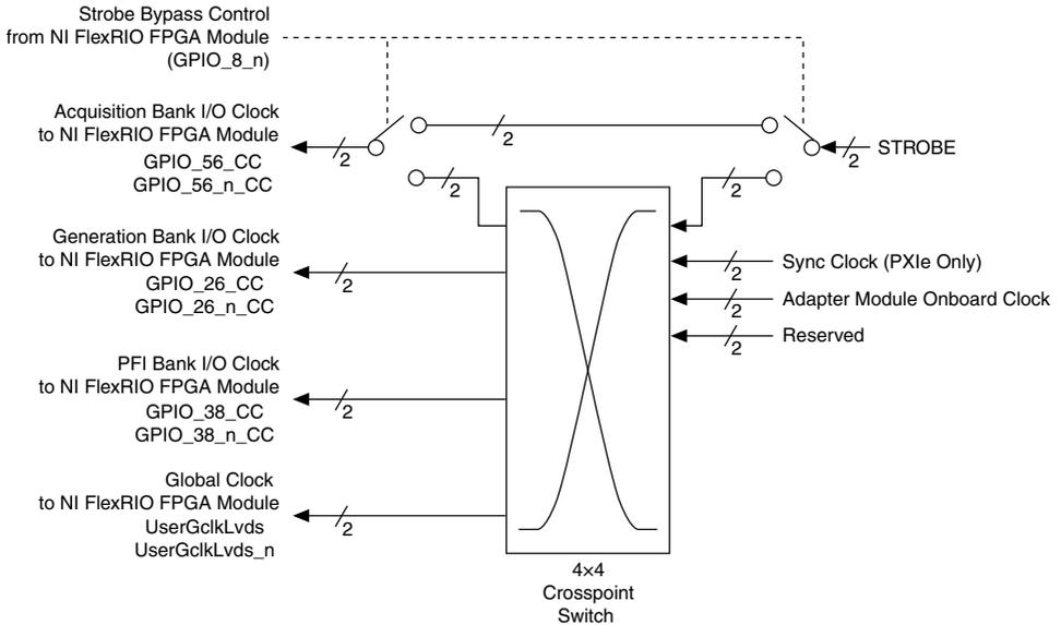
In software, each clock output terminal is accessed with a U8 data type. The following table shows the values of the crosspoint switch clock options.
