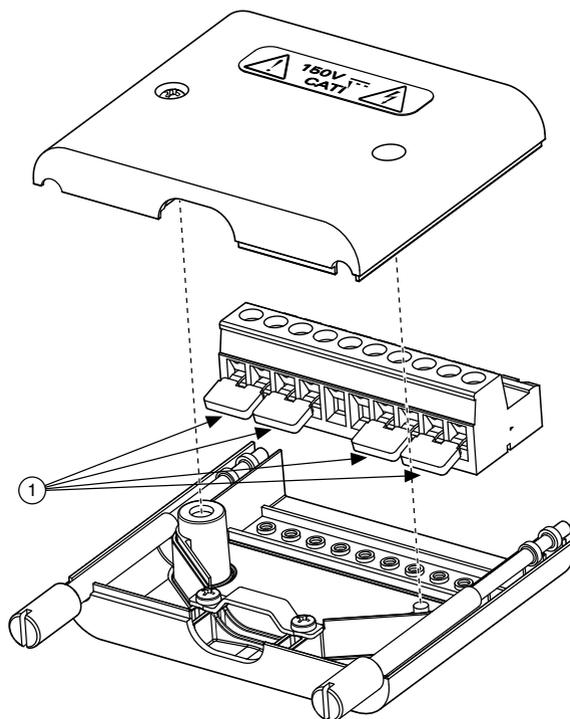
1. Sense Jumpers Installed on the Output Connector Plug
