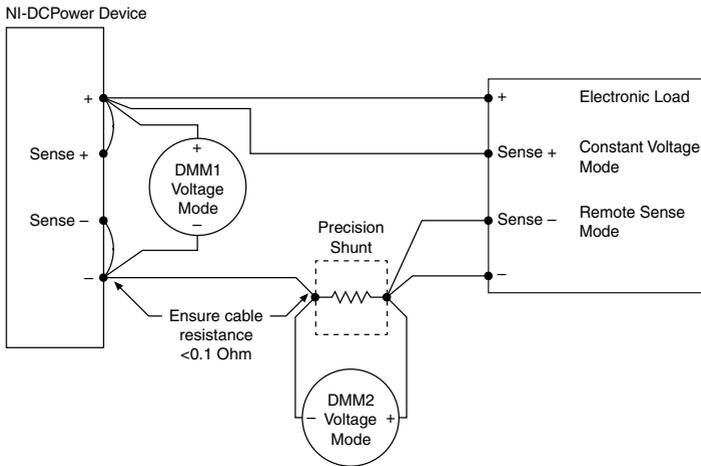
2. Connect the DMM to the NI 4113 connector pins with dedicated pairs of wires to avoid including lead drop in the DMM measurement.
