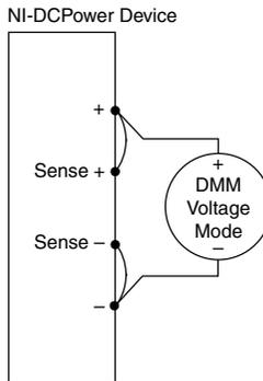
2. Set the **niDCPower Output Function** property or `NIDCPOWER_OUTPUT_FUNCTION` attribute to DC Voltage for the NI 4113.
