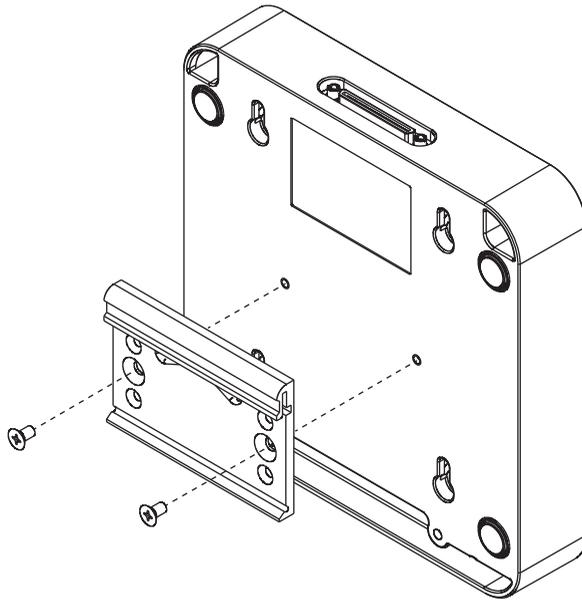
Clip the chassis onto the DIN rail with the larger lip of the DIN rail clip positioned up, as shown in Figure 4.
