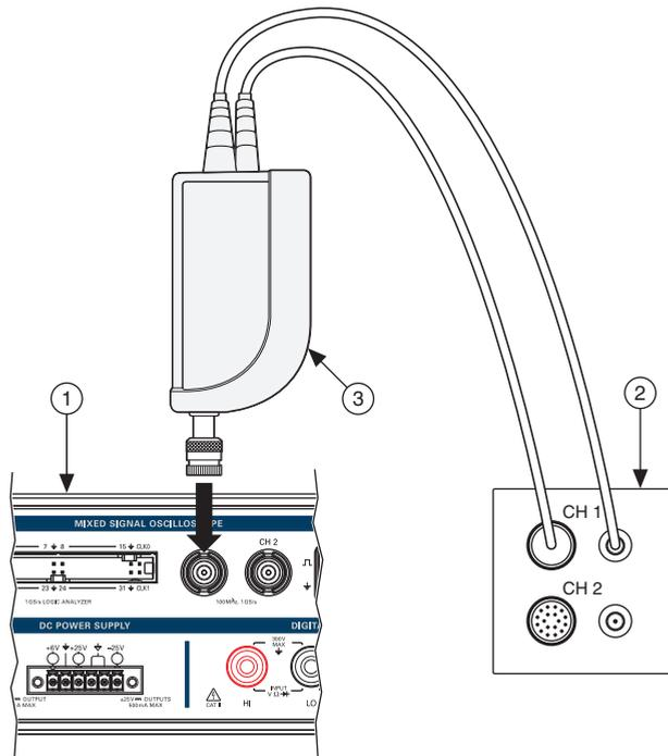
1 VirtualBench Oscilloscope 2 Oscilloscope Calibrator 3 Oscilloscope Calibrator Active Head
