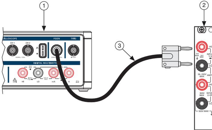
1 VirtualBench FGEN                      2 DMM                      3 Banana Plug-to-BNC Cable
