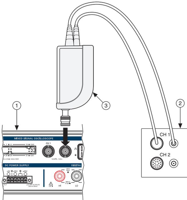
1 VirtualBench Oscilloscope 2 Oscilloscope Calibrator 3 Oscilloscope Calibrator Active Head
