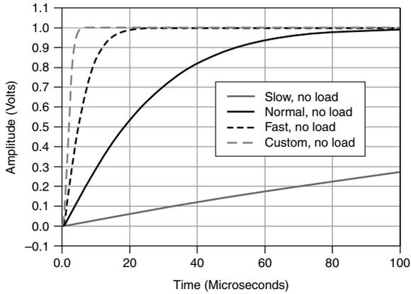
**Figure 8. 1 mA Range, 100 nF Load Step Response, Nominal**
