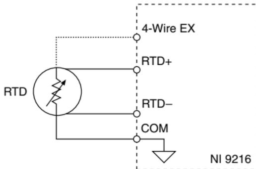
For the best measurement results when using the NI 9216 with a 3-wire RTD, use equal-length wires between the RTD+ terminal and the RTD and between the COM terminal and the RTD. Also, keep the lead resistance within 5% of the nominal RTD value. The NI 9216 accuracy specifications account for this lead error.
