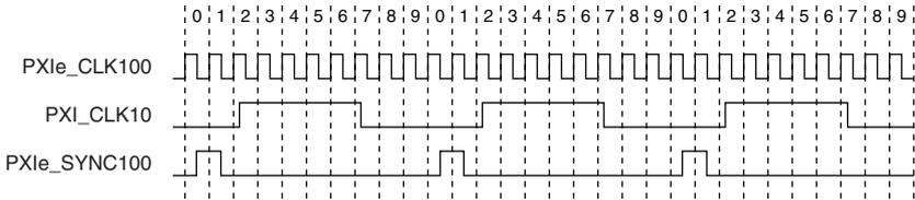
This architecture has the advantage that PXI\_CLK10 and PXIe\_CLK100 are always sourced from the same reference oscillator, and therefore it is impossible to lose PXI\_CLK10 or PXIe\_CLK100 by disconnecting a reference provided on any of the supported inputs. For the same reason, it is also impossible for a runt pulse or glitch to occur on these lines as references are switched in and out, protecting the integrity of digital circuitry operating on these clocks.
