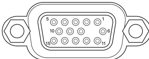
You can use a digital voltmeter to ensure all voltage levels in the chassis are within the allowable limits. Referring to Table 2-5, connect one lead of the voltmeter to a supply pin on the 15-pin remote voltage monitoring connector on the rear panel. Connect the reference lead of the voltmeter to one of the ground pins. Compare each voltage reading to the values listed in Table 2-6.
