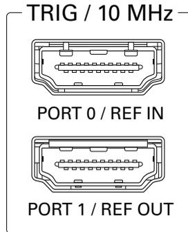
Routing triggers between chassis requires using a National Instruments API such as NI-DAQmx. You can target the individual pins of each trigger port as sources or destinations for PXI triggers to or from a PXI module. If the chassis are connected to the same host via MXI, then targeting these pins is not necessary; you can specify a source device in one chassis and a destination device in another chassis and the software will make the necessary trigger routes automatically.
