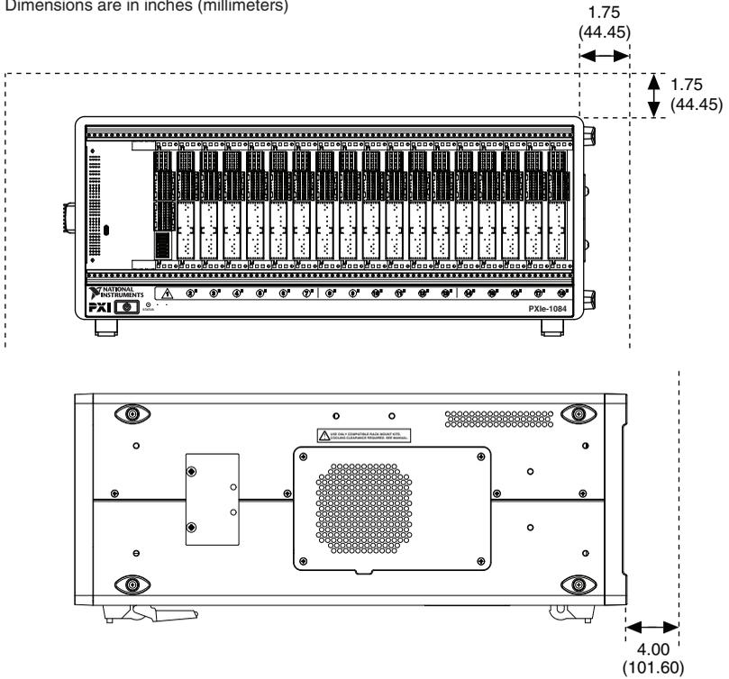
Figure 2-2. PXIe-1084 Chassis Vents
