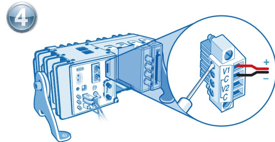
Connect the positive lead of the power source to the V1 terminal on the power connector plug, and the negative lead to one of the C terminals.
