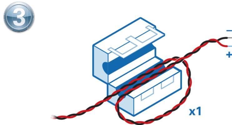
Verify power source is turned off. Install ferrite across the negative and positive leads of the power source.
