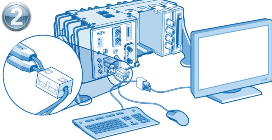
Connect a computer keyboard and mouse with ferrite and a monitor to the cDAQ controller.
