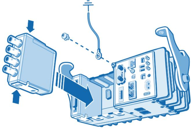
Connect the cDAQ controller to earth ground. Then install I/O modules. Refer to the module operating instructions for signal connections.
