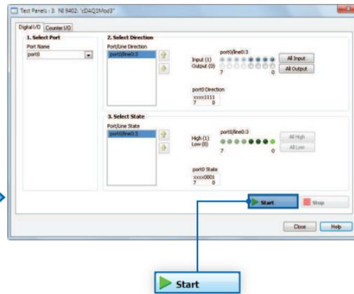
Take your first measurement in MAX. Right-click any module and select **Test Panels**. Configure the measurement settings and click **Start**.
