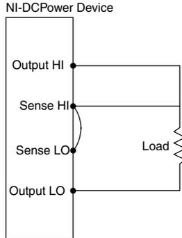
3. Set the **niDCPower Output Function** property or `NIDCPOWER_OUTPUT_FUNCTION` attribute to DC Current for the PXIe-4162/4163.
