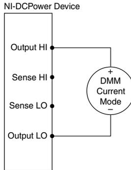
2. Set the first specified level range, limit range, and limit on the PXIe-4162/4163.
