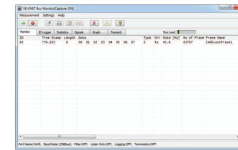
In Measurement & Automation Explorer (MAX), right-click the CAN interface under the device and select Bus Monitor. After selecting network parameters, click the start button to verify functionality.
