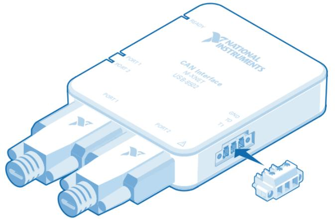
**Optional:** Attach the synchronization connector plug to the device.
