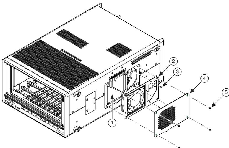
1. Chassis Side Fan Cavity
