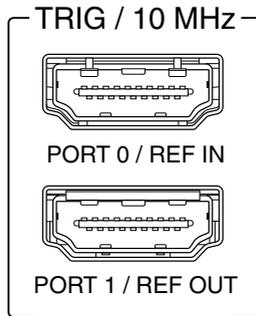
Routing triggers between chassis requires using a National Instruments API such as NI-DAQmx. You can target the individual pins of each trigger port as sources or destinations for PXI triggers to or from a PXI module. If the chassis are connected to the same host via MXI, targeting these pins is not necessary; you can specify a source device in one chassis and a destination device in another chassis, and the software makes the necessary trigger routes automatically.
