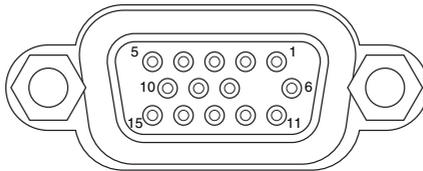
You can use a digital voltmeter to ensure all chassis voltage levels are within the allowable limits. Referring to the previous table, connect one voltmeter lead to a supply pin on the 15-pin remote voltage monitoring connector on the rear panel. Connect the voltmeter reference lead to one of the ground pins. Compare each voltage reading to the values in the following table.
