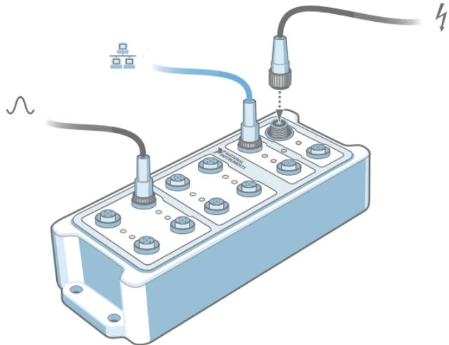
Connect Ethernet Port 0 on the FieldDAQ to a network port or directly to the network card in your computer. Then connect the power supply to the Power IN Port.
