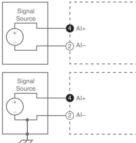
Connect signals to the FieldDAQ. Refer to the user guide for complete signal connection information.
