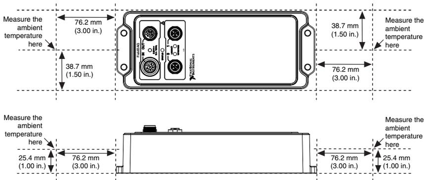
**Figure 27. Ambient Temperature Locations, Vertical Mounting Configuration**
