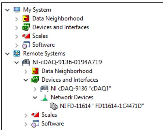
11. If the FieldDAQ device is not reserved automatically, select the device and click the **Reserve Network Device** button. Refer to [Reserving the Device in MAX](#) for more information.
