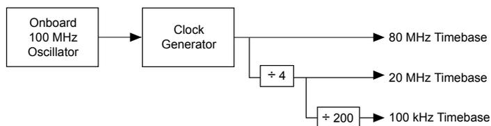
You can use the 80 MHz, 20 MHz, and 100 kHz timebases to generate the measurement signals. The 80 MHz timebase is generated directly from the onboard clock generator. The 20 MHz and 100 kHz timebases are generated by dividing down the 80 MHz timebase.
