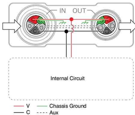
The FieldDAQ device requires an external power source connected between the V and C terminals, as described in *Power Requirements* in the *FD-11614 Specifications*. The FieldDAQ
