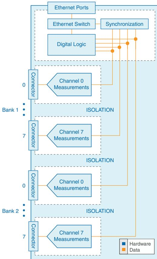
The FD-11614 provides channel-to-channel isolation.
