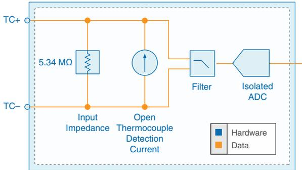
**Figure 9.** FD-11614 Block Diagram
