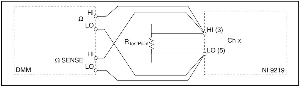
**Figure 6.** Quarter-Bridge Accuracy Verification Connections to the NI 9219
