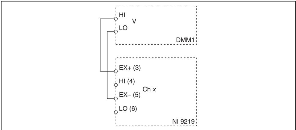
**Figure 15.** Full-Bridge Accuracy Verification Connections to the NI 9219 (Configuration 1)
