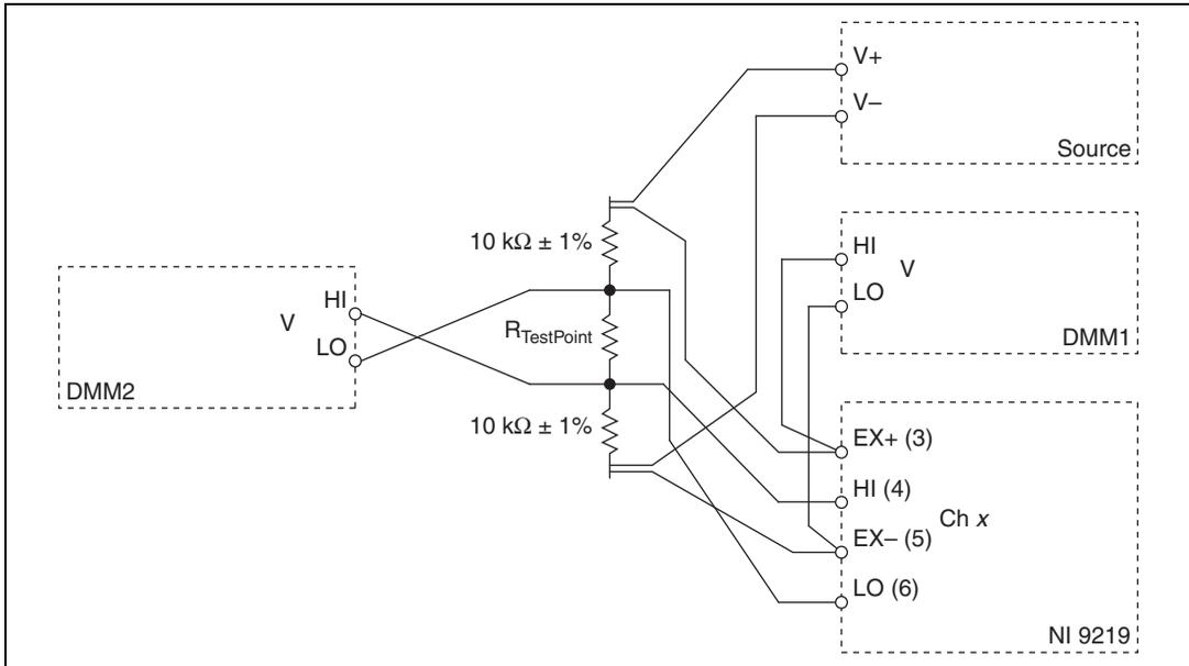
**Figure 17.** Full-Bridge Accuracy Verification Connections to the NI 9219 (Configuration 3)
