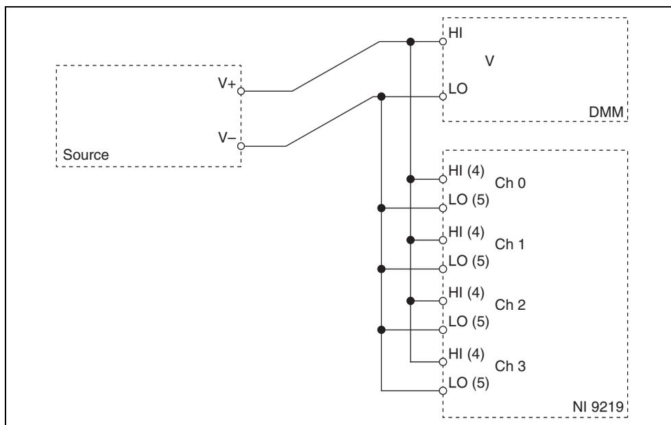
**Figure 2.** Voltage Accuracy Verification Connections to the NI 9219
