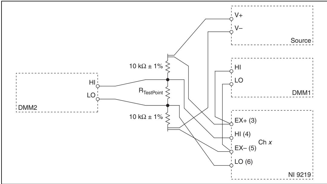
**Figure 16.** Full-Bridge Accuracy Verification Connections to the NI 9219 (Configuration 2)
