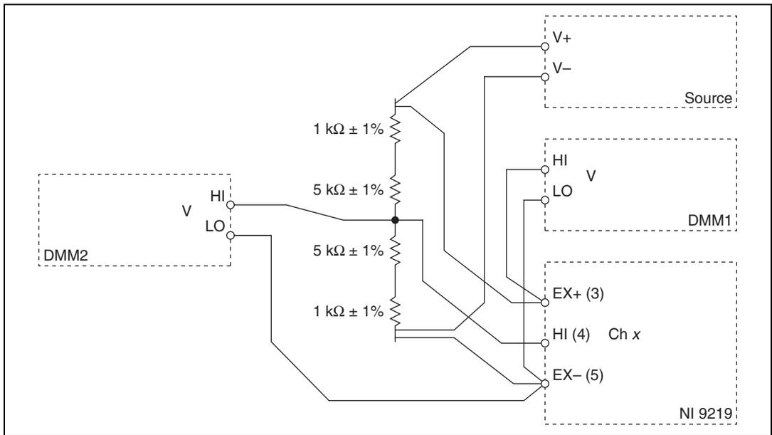
**Figure 13.** Half-Bridge Accuracy Verification Connections to the NI 9219 (Configuration 3)
