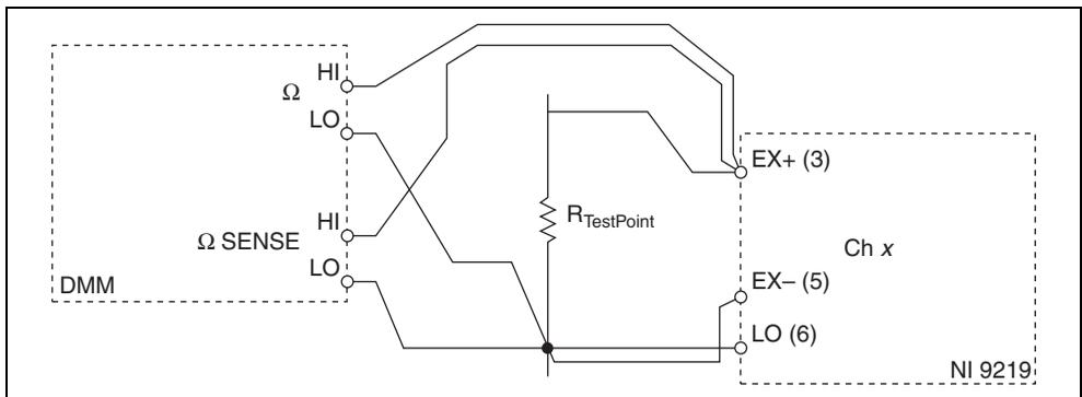
**Figure 9.** 3-Wire RTD Accuracy Verification Connections to the NI 9219
