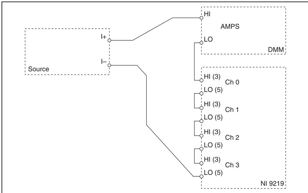
**Figure 4.** Current Accuracy Verification Connections to the NI 9219
