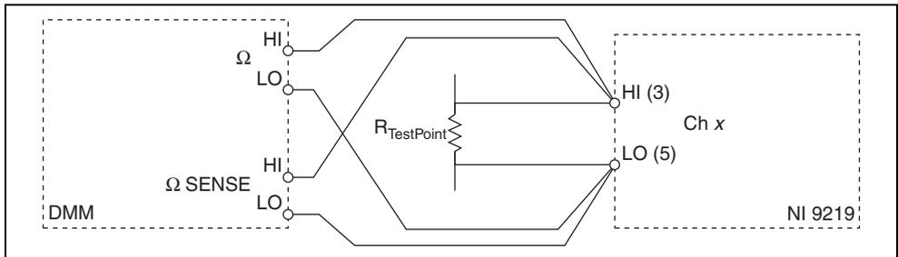
**Figure 5.** 2-Wire Resistance Accuracy Verification Connections to the NI 9219
