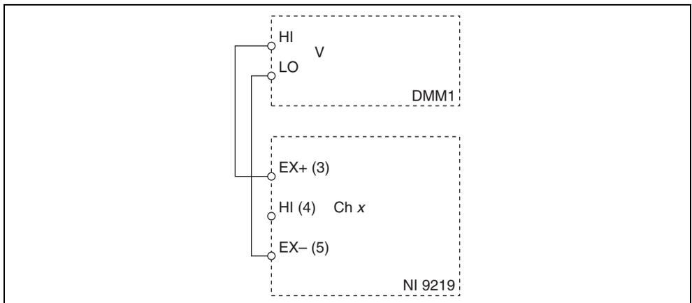
**Figure 11.** Half-Bridge Accuracy Verification Connections to the NI 9219 (Configuration 1)
