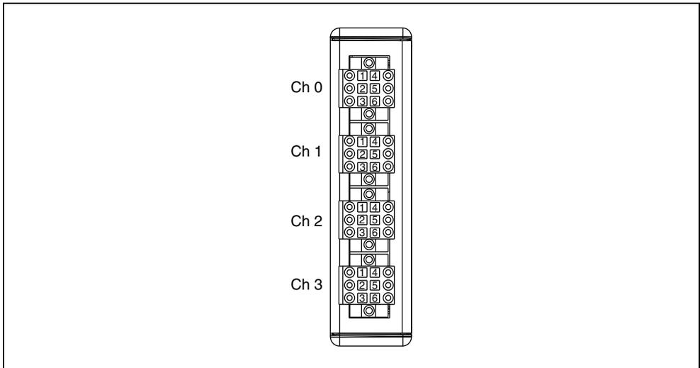
**Figure 1.** NI 9219 Channel and Terminal Assignments
