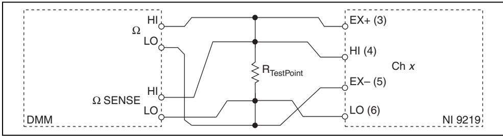
**Figure 8.** 4-Wire RTD Accuracy Verification Connections to the NI 9219
