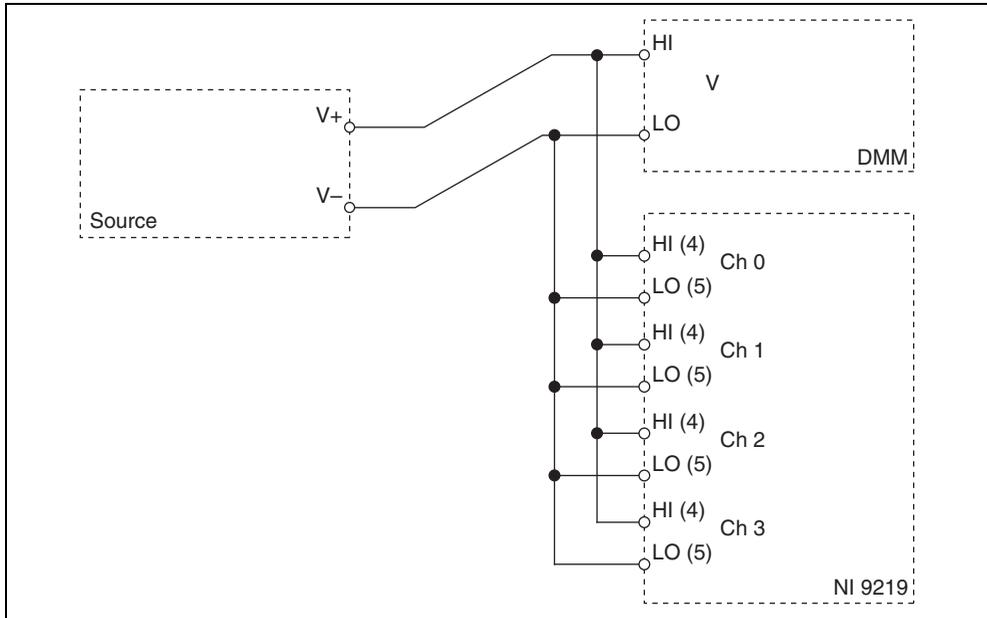
**Figure 3.** Thermocouple Accuracy Verification Connections to the NI 9219
