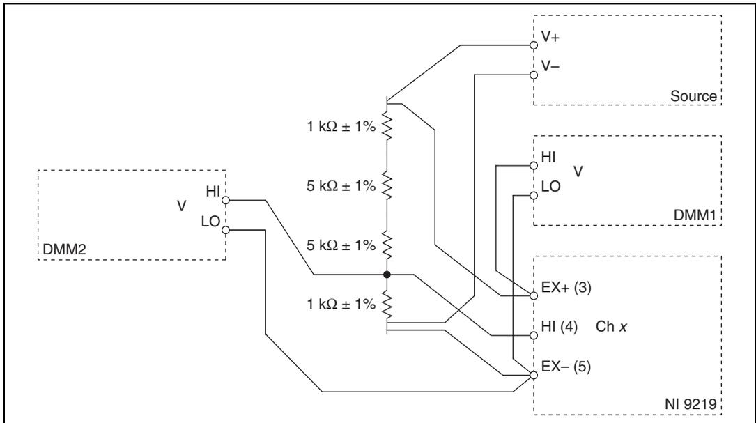
**Figure 14.** Half-Bridge Accuracy Verification Connections to the NI 9219 (Configuration 4)
