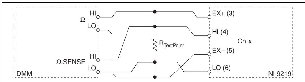
**Figure 7.** 4-Wire Resistance Accuracy Verification Connections to the NI 9219
