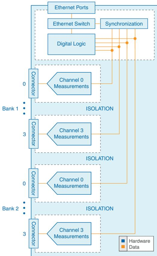
The FD-11601 provides channel-to-channel isolation. Input signals on each channel are conditioned, buffered, and then sampled by an ADC. Each AI channel provides an independent signal path and ADC, enabling you to sample all channels simultaneously. The FieldDAQ device provides overvoltage protection for each channel; refer to the *FD-11601 Specifications* for more information about overvoltage protection.
