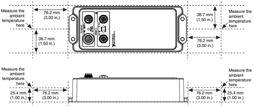
**Figure 35. Ambient Temperature Locations, Vertical Mounting Configuration**
