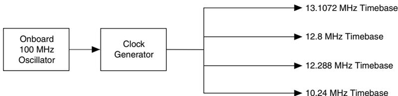
You can use the 13.1072 MHz, 12.8 MHz, 12.288 MHz, and 10.24 MHz timebases to generate the AI Sample Clock signals. These timebases are generated directly from the onboard clock generator. By default, NI-DAQmx automatically chooses the most suitable timebase for a selected data rate. You can also manually select a timebase through the NI-DAQmx API.
