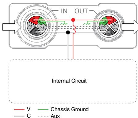
The FieldDAQ device requires an external power source connected between the V and C terminals, as described in *Power Requirements* in the *FD-11601 Specifications*. The FieldDAQ
