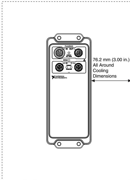
Allow the appropriate space in front of the device for cabling clearance, as shown in the following figure.
