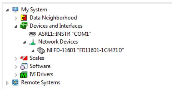
9. If the FieldDAQ device is not reserved automatically, select the device and click the **Reserve Network Device** button. Refer to [Reserving the Device in MAX](#) for more information.
