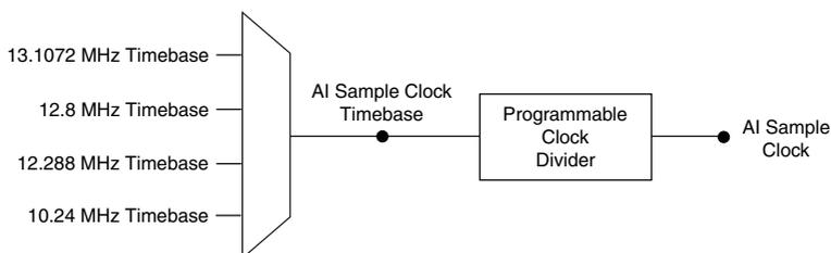
The FD-11601 is considered a Delta-Sigma device; it contains multiple A/D converters that require a high-frequency oversample clock to produce accurate, synchronized data. The FieldDAQ device returns a sample on every Sample Clock pulse.
