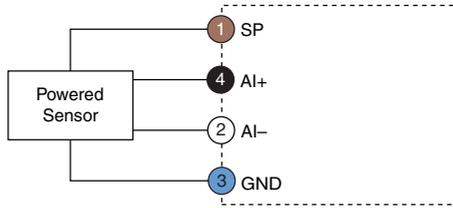
**Figure 14. Powering a 3-Wire External Sensor**
