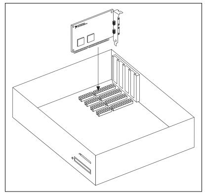
Figure 2-5. AT Serial Board Installation
