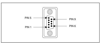
Figure 2-8. DB-9 Connector Pin Locations
