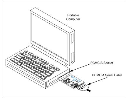
Figure 2-4. Inserting a PCMCIA Serial Card
