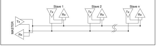
Figure B-2. Typical Half-Duplex System
