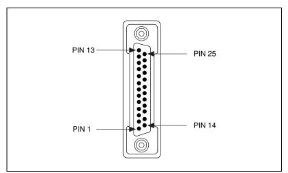
Figure 2-10. DB-25 Connector Pin Locations
