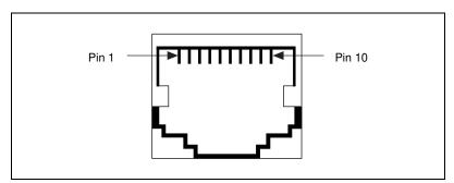
Figure 2-9. 10-Position Modular Jack Pin Locations
