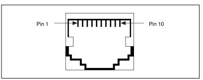
Figure 2-6. 10-Position Modular Jack Pin Locations
