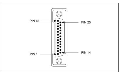
Figure 2-7. DB-25 Connector Pin Locations
