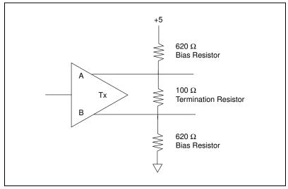
Figure B-4 shows a transmission line using bias resistors.
