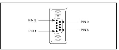
Figure 2-5. DB-9 Connector Pin Locations
