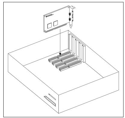
Figure 2-4. AT Serial Board Installation
