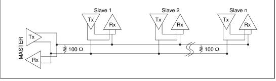
Figure B-3. Multidrop Network Using Terminating Resistors
