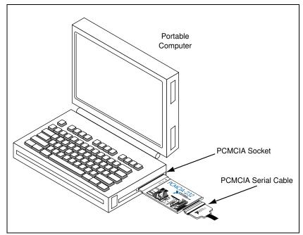
Figure 2-3. Inserting a PCMCIA Serial Card
