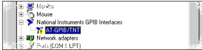
Figure 2-14. GPIB Interface That Is Not Working Properly
