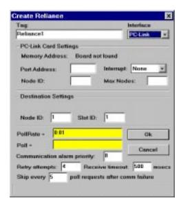
Note If you are developing your application without a PC-Link card installed in your computer, and do not know the settings that in the target system, you can enter 250 for Port Address, 0 for Node ID, and 3 for Max Nodes. You can then create the Reliance object and correct the parameter values for the actual system later, if necessary.
