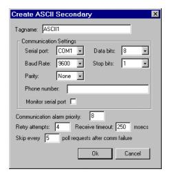
**Serial port** specifies which COM port the object uses for communicating to the external device. This does not specify the communication type. Communication type is determined by the Options—Serial Ports... command.
