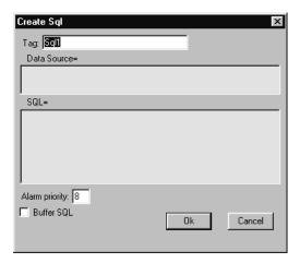
**Data Source** specifies the Data Source Name (DSN) as well as any other parameters needed by the ODBC driver to make the connection to the data source. For example if you want to connect to Excel 4.0, use
