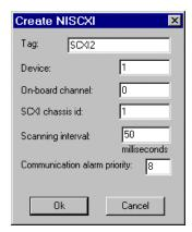
**Device** is the NI-DAQ device number of the controlling device. The DAQ configuration utility (WDAQConf.exe) assigns this number to an installed device. Valid device numbers range is from 1 to 16.
