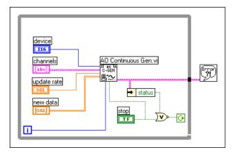
Figure 12-4. Circular Buffered Waveform Generation Using the AO Continuous Gen VI
