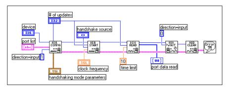
Figure 17-7. Reading Data with the Digital VIs Using Digital Handshaking (DIO-32 Series Devices)
