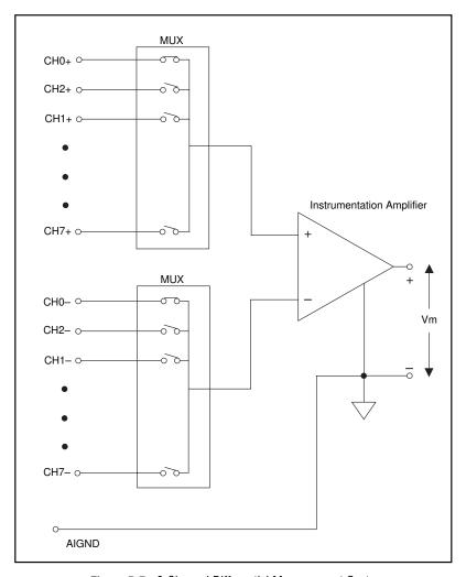
Figure 5-7. 8-Channel Differential Measurement System
