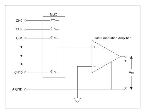
**Figure 5-9.** 16-Channel RSE Measurement System
