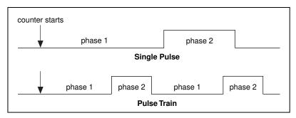
Figure 24-3. Pulses Created with Positive Polarity and Toggled Output
