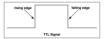
Figure 9-3. Example of a TTL Signal
