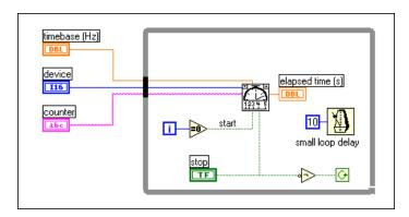
Figure 27-10. Diagram of Count Time-Easy (DAQ-STC) VI
