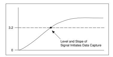
Figure 8-4. Diagram of an Analog Trigger
