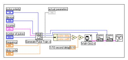
Figure 24-18. Diagram of Finite Pulse Train-Easy (DAQ-STC) VI
