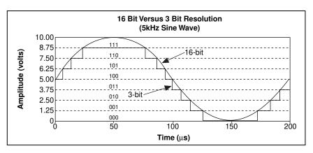
**Figure 5-4.** The Effects of Resolution on ADC Precision
