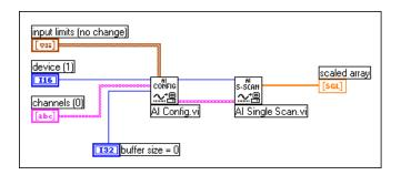
**Figure 6-5.** Using the Intermediate VIs for a Basic Non-Buffered Application
