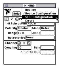
Figure 2-6. Accessing the NI-DAQ SCXI Configuration Window
