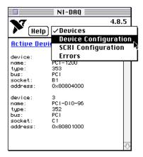
Figure 2-4. Accessing the Device Configuration Window in NI-DAQ
