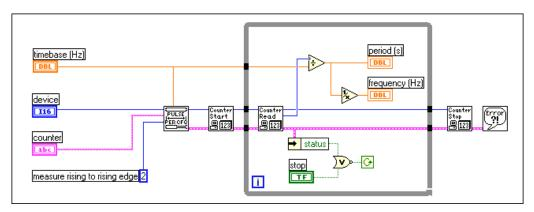
Figure 26-11. Measuring Period Using Intermediate Counter VIs
