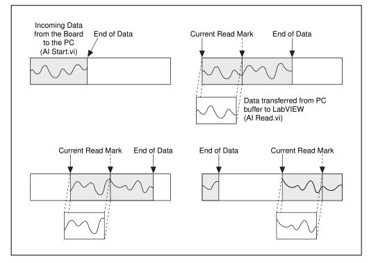
Figure 7-9. How a Circular Buffer Works
