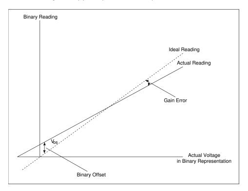
In this picture, you can see the difference between the ideal reading and the actual reading. This difference is called  $V_{os}$ , or the **binary offset**, before the two readings intersect. The difference in slope between the actual and ideal readings is called the **gain error**.
