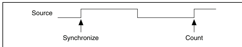
Figure 7-35. 80 MHz Source Mode
