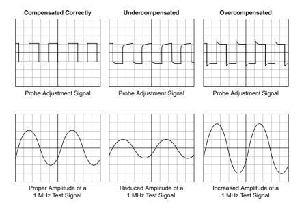
Once compensated, the probe conveys signals to the input channel accurately, without artificially attenuating or amplifying frequency components of the signal.
