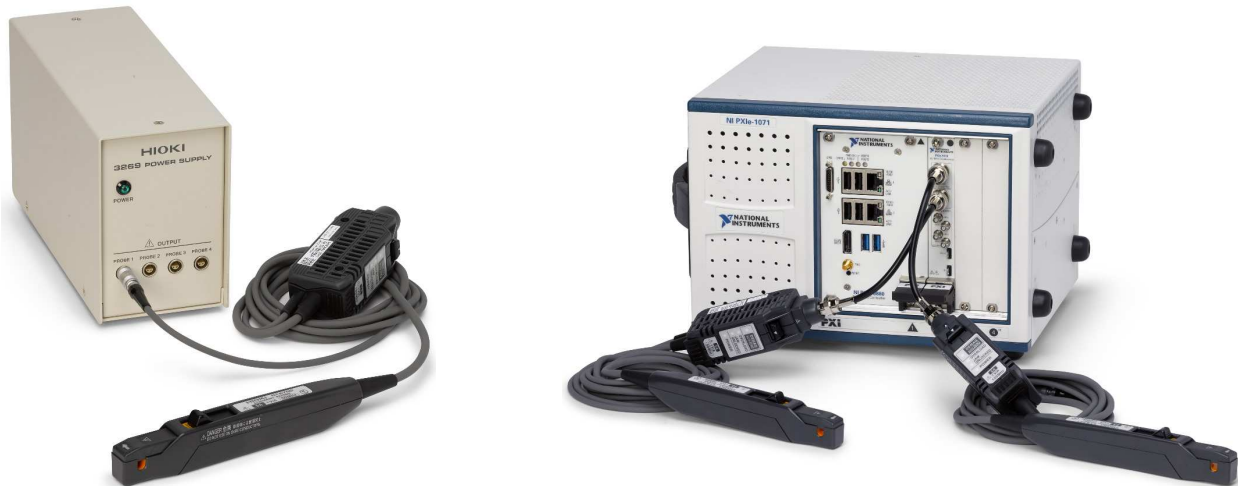
Figure 1. Hioki current probes require power supplies and also may need short cable adapters if using with SMA/SMB scopes or BNC scopes with closely adjacent channels.
