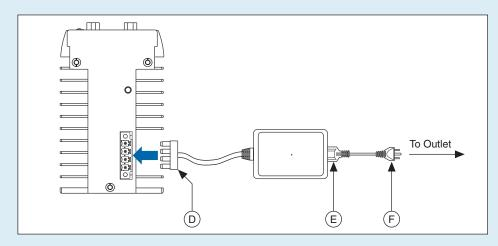
D. Plug the 4-position connector from the power supply into the power receptacle on the NI CVS-1450 device.
