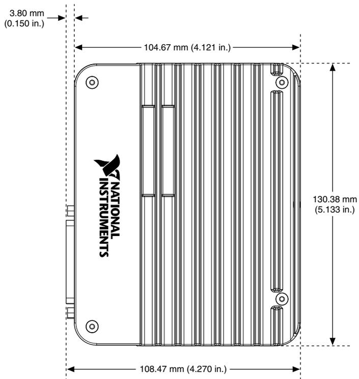
**Figure 22. Bottom View with Dimensions in inches [millimeters]**
