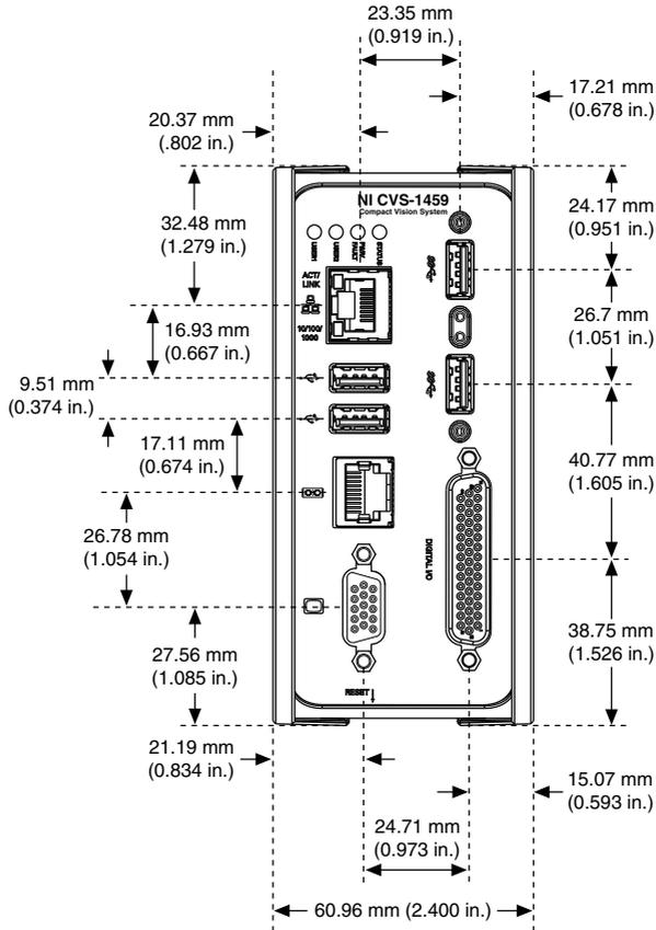
**Figure 20. Back View with Dimensions in inches [millimeters]**
