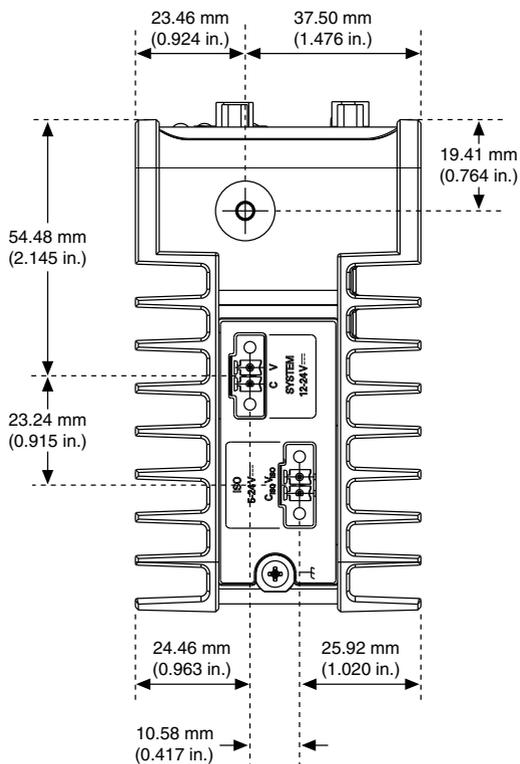
**Figure 21. Side View with Dimensions in inches [millimeters]**
